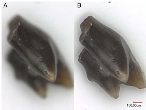
Fig. 2. Illustration of in-focus z-series reconstruction system which corrects the problems of depth of focus on stereomicroscope. Dryolestidae mammalian tooth (CHEM03.587, mesiolingual view, Berriasien, Cherves-de-Cognac, Charente, France) performed on a digital microscope Keyence VHX-600. A: Focus for a single image (classical stereomicroscope picture). The problem of depth of focus results in a blurring at the background outline of the tooth. B: Result of the compilation of in-focus planes on the whole depth of the tooth.
